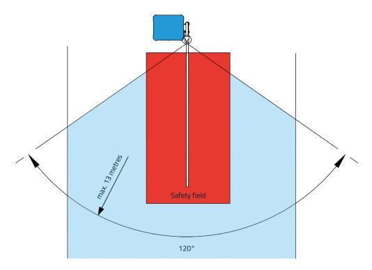
Installation under the barrier boom, e.g. for the exclusive safety function or as a loop replacement.
