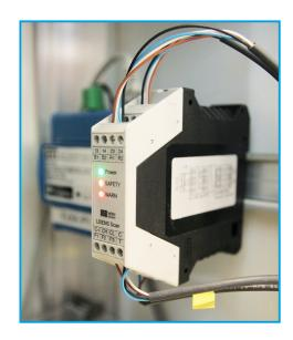
With a total of four relay outputs, the radar Comfort has an additional relay for the safety field.
