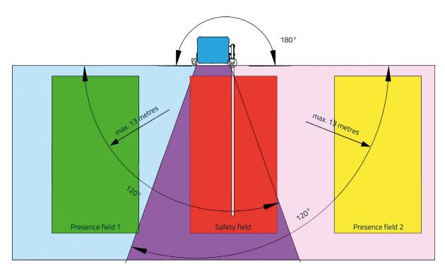
Mounting with 2 sensors (monitoring angle extended to 180°) e.g. for protection and vehicle detection on both sides.
