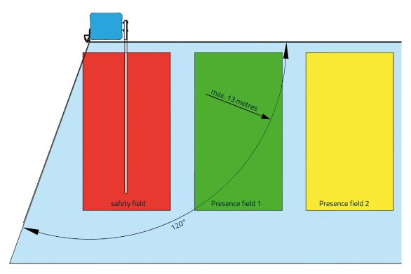
Mounting opposite the barrier boom, e.g. for protection and vehicle detection. Presence fields can be combined for directional logic.
